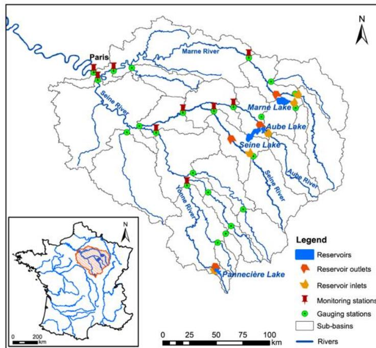
Figure 3 Main river network, reservoirs and gauging and monitoring stations of the Seine River<sup>36</sup>
